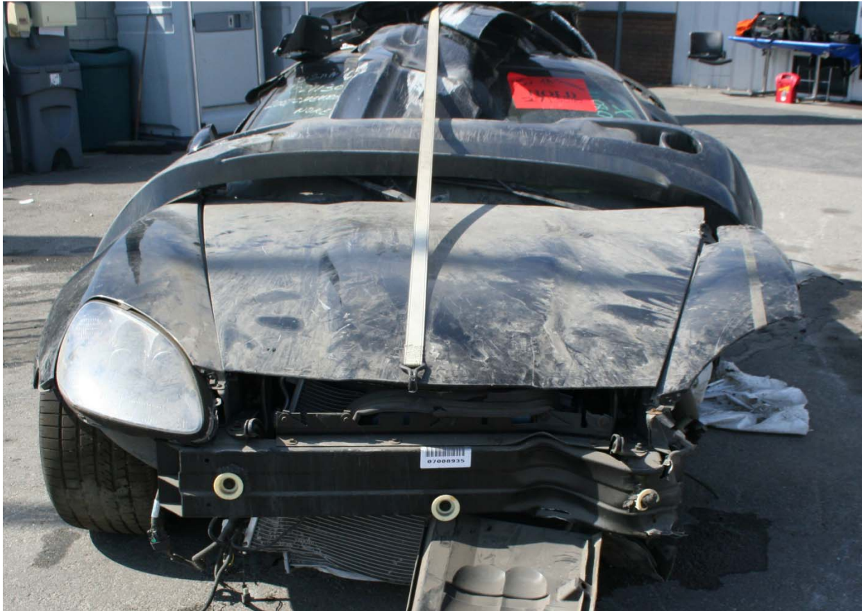
Figure 7. Collision damage resulting in air bag deployment.
