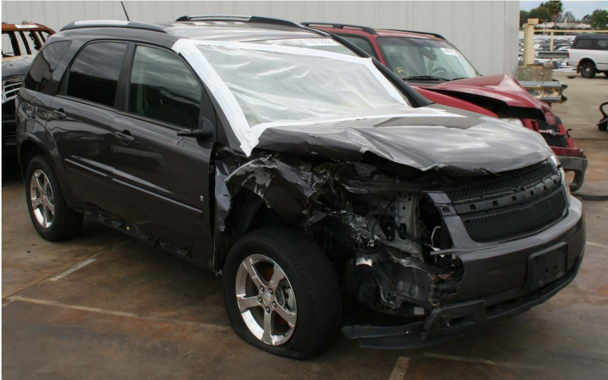
Figure 6. Collision damage resulting in non-deployment of front passenger/driver air bags.
